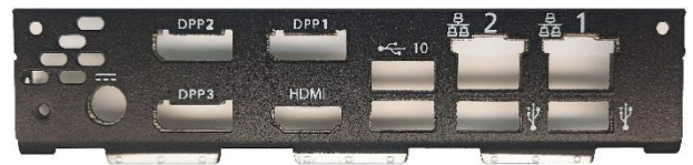
Chassis rear wall (K1056-B622) with 4 x graphics
