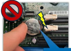
Do **not** insert battery on the plastic clips side at first!
