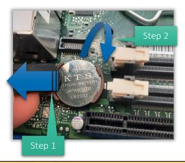
Note: The bracket is very sensitive. Ensure not to bend the metal part. Otherwise contact issues can occur.
