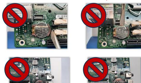
This could damage the solder pads, metal brackets or plastic noses. These leads to malfunction of the battery contact -> RTC reset or BIOS battery voltage error message.
