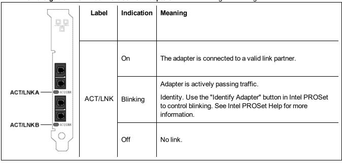
The Intel® **PRO/1000 MF**, **PF**, and **Gigabit EF Dual Port Server Adapters** have the following indicator lights for each port:
