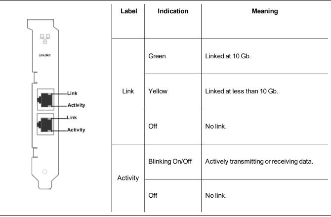
The Intel® Ethernet Server Adapter I350-T2, I340-T2, PRO/1000 P, PT Dual Port, and Gigabit ET Dual Port Server Adapters have the following indicator lights:
