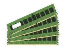
\*) These modules are fully approved for motherboard version D3598-B14 (8 layer design)! Modules may fail if used in memory channel "D" of previous motherboard versions
