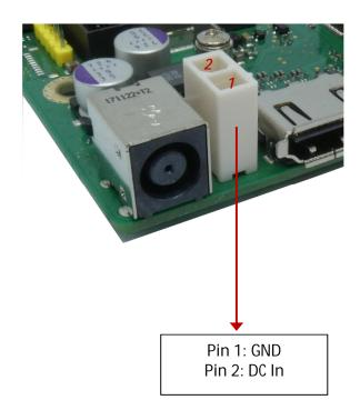
Internal and external DC input can be powered by 19-24V (+10% / -15%).
