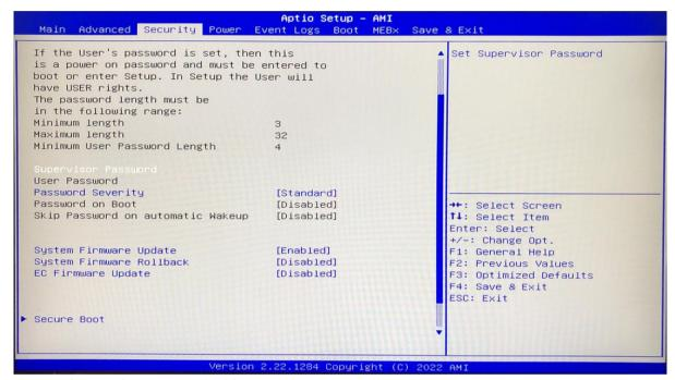
Figure 3: Security Setup Menu Initial Screen
